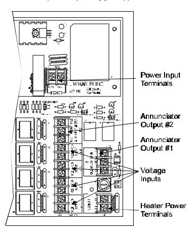
Figure 3-9: I/O Board Terminal Locations
